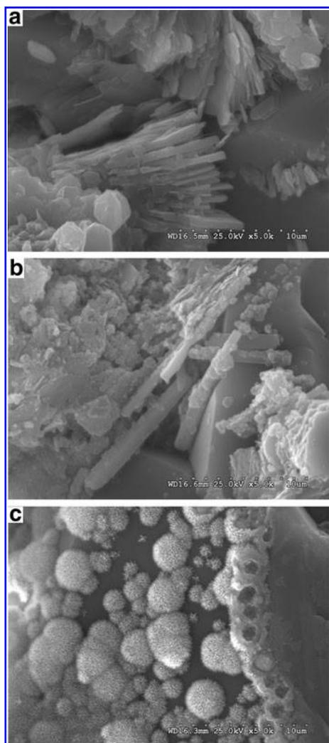
**FIG. 6.** (a) SEM image of numerous hexagonal plates of iron-oxide cement filling pore space between quartz sand grains. (b) SEM image of iron-oxide cement comprising hexagonal plates and lath-like mineral grain (in lower center of image). Note the late-stage clumps of acicular grains occurring as an overgrowth on all other forms of iron oxide. (c) SEM image of hemispherical aggregates of iron-oxide needles on a quartz grain.
