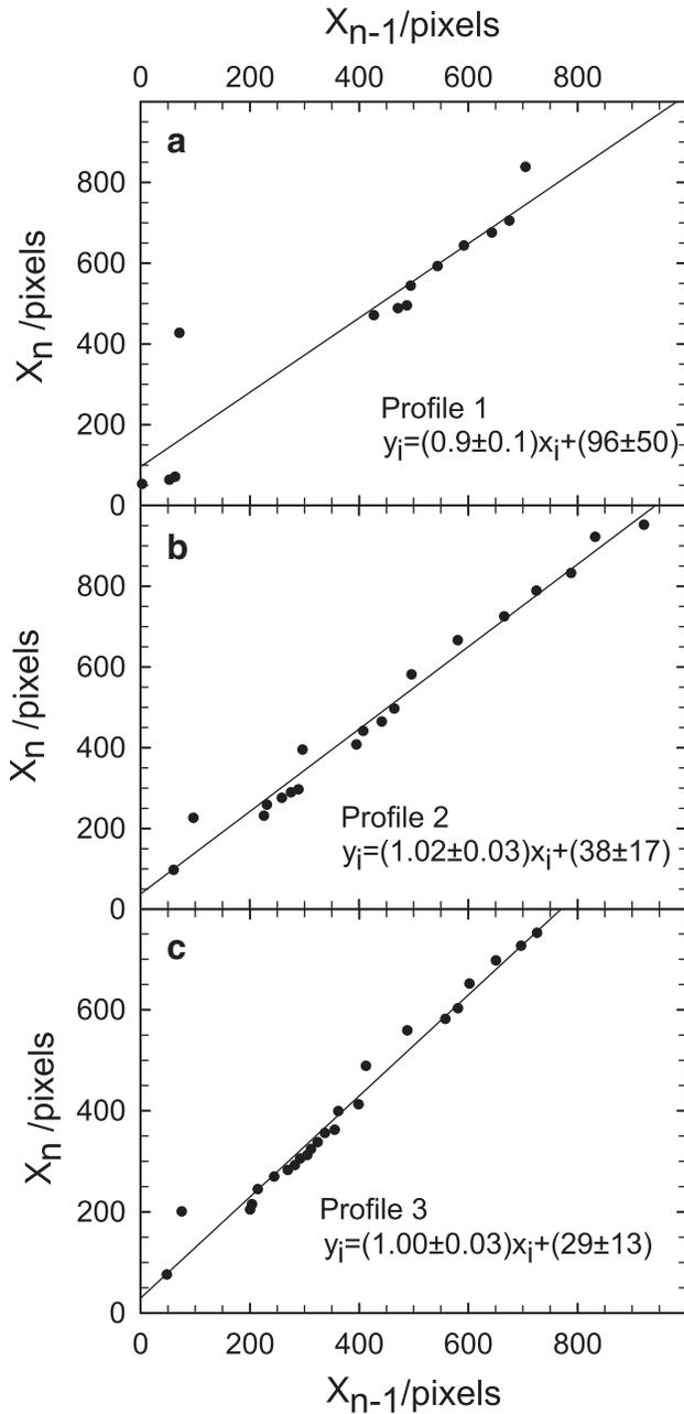
**FIG. 10.** (a–c) Results of tests of spacing law for profiles taken on Image P3180044 (Fig. 3), Profiles 1–3, respectively. All regressions of  $X_n$  on  $X_{n-1}$  yield slopes equal to unity.
