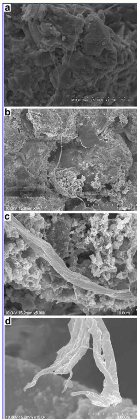
**FIG. 7.** (a) SEM image of numerous twisted filaments cemented to quartz grains and covered locally by IOC. (b) Image of long twisted filament anchored to iron-oxide cement at top of image. (c) Detailed SEM image of portion of feature shown in (b) illustrating the number of filaments in the stalk, the twisted nature of the stalk, and the relationship to IOC. (d) Detailed SEM image of the free end of stalk shown in (b) and (c).
