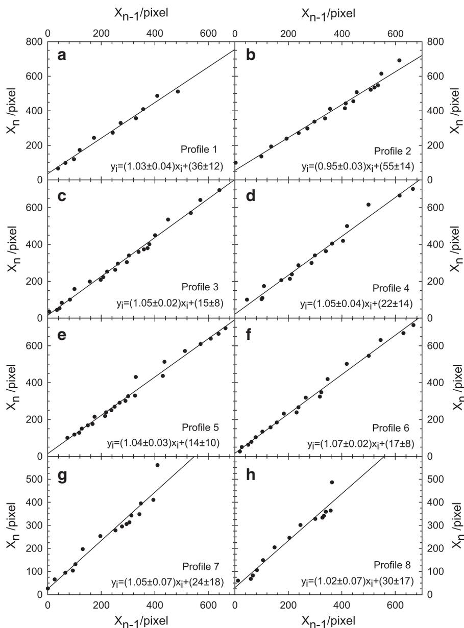
**FIG. 11.** (a–h) Results of tests of spacing law for profiles taken on Image P3190192 (Fig. 4), Profiles 1–8, respectively. All regressions of  $X_n$  on  $X_{n-1}$  yield slopes equal to or very close to unity.
