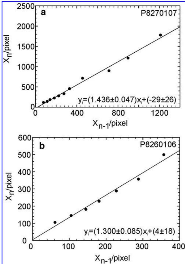
**FIG. 12.** (a) Results of test of spacing law for profile taken in Image P8270107 (shown in Fig. 5a) and (b) Image P8260106 (shown in Fig. 5b and 5c). Both profiles yield slopes greater than 1 with values that are consistent with the Jablczynski spacing law (Antal *et al.*, 1998). Scale for Image P8270107 is 60 pixel/mm, whereas scale for Image P8260106 is 75.2 pixel/mm.
