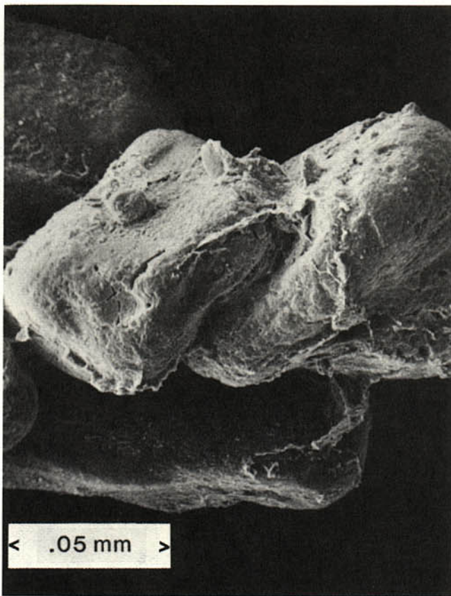
FIGURE 7 —SEM image of sand grains with detrital clay coatings and bridges. Sample is a “crumb” of recently deposited, but cohesive surface sand collected from the side of a vertical-sided cow track in the central Sand Hills.
